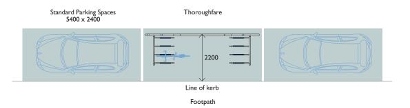
$\begin{tabular}{lll} \textbf{Material Specifications (General)} \\ \textbf{Rack} & 50 \times 50 \text{ SHS Mild Steel / 25NB } \times 1.5 \text{mm Pipe / Galvanised} \\ \textbf{Profile} & 65 \text{NB (76.1)} \times 3.6 \text{mm pipe / Galvanised} \\ \end{tabular}$
